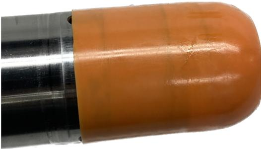
**#2 Use a seal bullet tool to install seals onto the fork tube.**
