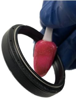
**#1 lightly grease ID and OD of seals before installation.**
