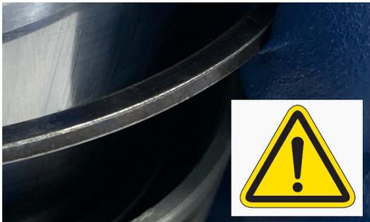
**#7 Install wire ring into wire ring groove and double check to make sure it seated properly into groove. You can use a small flat screw driver or pick to do so.... this is very important !!**
