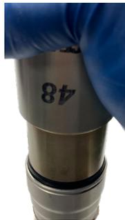
**#6 Use seal driver and strike the seal a few times to press it to the bottom of the seal housing. Make sure then seal is below the wire ring groove.**
