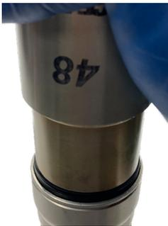
**#4 install inner fork tube into outer fork tube and slide bushings and spacer down into upper tube housing. It's a good practice to use the seal sitting driver to to set the bushing and spacer washer into tube housing.**
