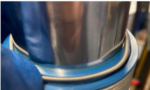
**#11** Pull the garter spring down and install the garter spring back onto dust wiper.
