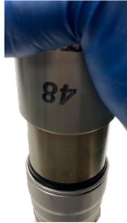
**#5 Push the oil seal down as far as you can into seal housing with seal drive tool to square seal up into housing bore.**
