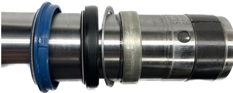
**#3 Remove seal bullet tool and install spacer washer and the two slide bushings onto fork tube.**
